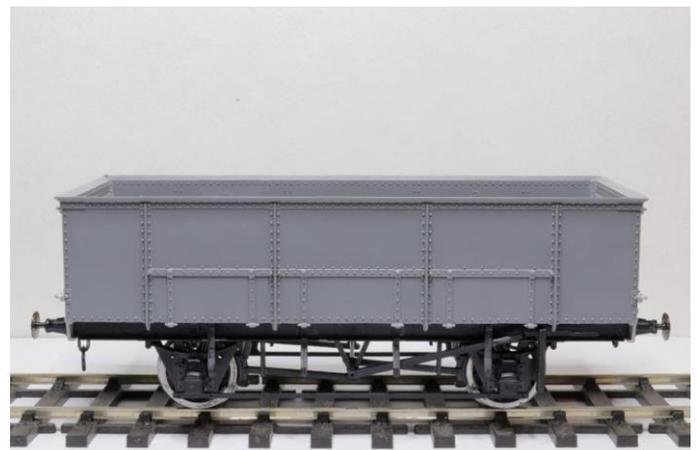
Following is the model painted with the chassis in a track colour brown and the body in a light freight grey. The image shows how I have painted the backs of the brake gear, wheels and axles. There are two reasons for this. Firstly, it prevents the wheels and axles rusting and secondly, close up photos with a camera and flash are always cruel: the flash always finds unpainted areas which should otherwise be painted.
