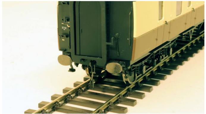
*Above: Brake end showing screw link coupling*
