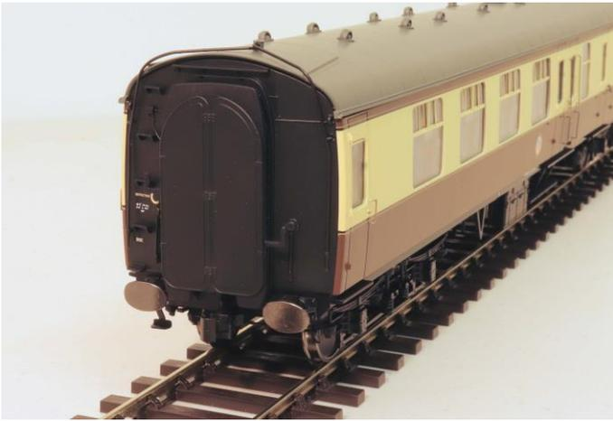
*Above: Passenger end showing buckeye coupling and BR round topped blanking board*
