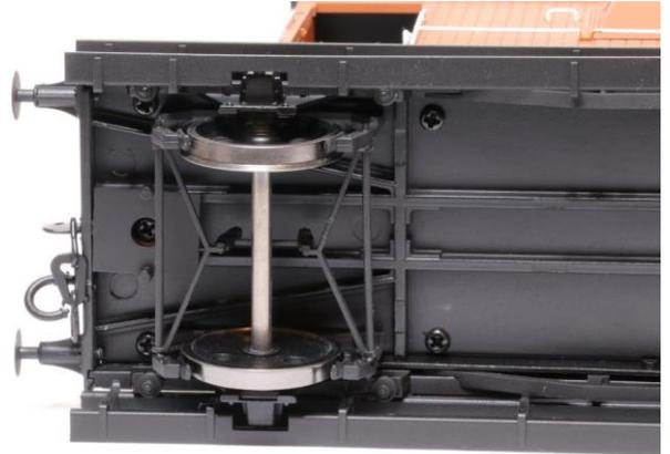
The wheels seem to run true. The compensation system would iron out minor discrepancies anyway.
