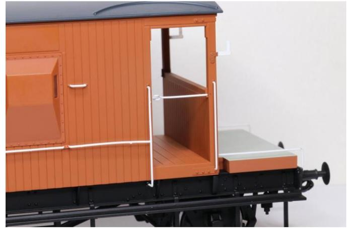
***The buffers are sprung as is the coupling hook, in this instance, fitted with instanter couplings. The vacuum brake pipe is also modelled.***
